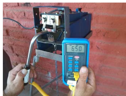
Pyrometer indicating proper blade temperature of 650°C.
